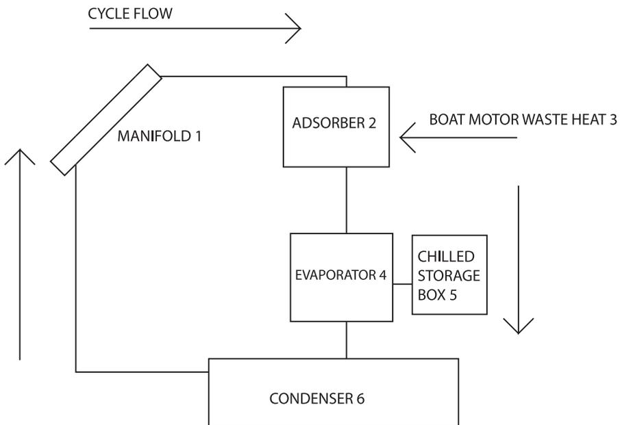
Figure 4. Description of the Closed Solar Adsorption Fridge Cycle.
