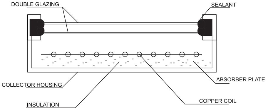
Figure 1. *Typical cross section of a flat plate solar collector.*
