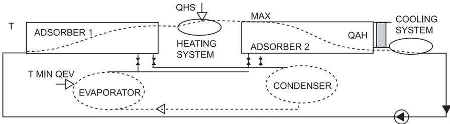
Figure 10. Presentation of the three main heat quantities that describe the process:  $Q_{EV}$  is the cold production at the evaporator;  $Q_{AH}$  is the heat quantity supplied to the adsorbers by the HX-fluid in the heating periods and  $Q_{HS}$  is the energy supplied by the heat source.
