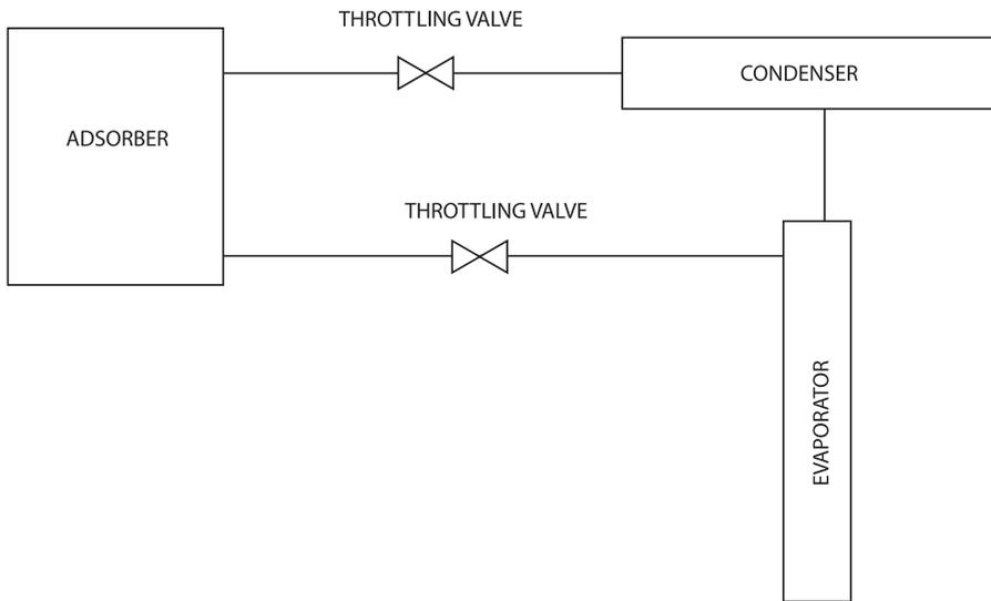
Figure 2. Schematic of a Basic Adsorption Cycle.
