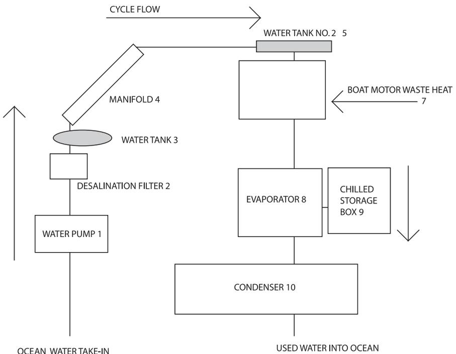
Figure 3. Description of the Open Cycle Solar Adsorption Fridge.
