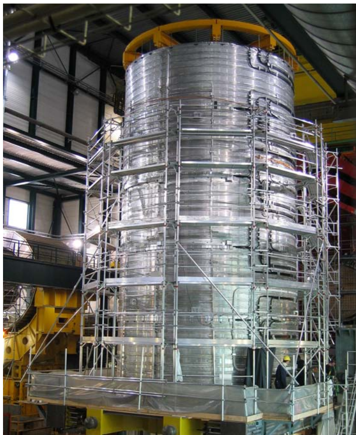
Figure 2.2: The cold mass mounted vertically before integration with thermal shields and insertion in the vacuum chamber.
