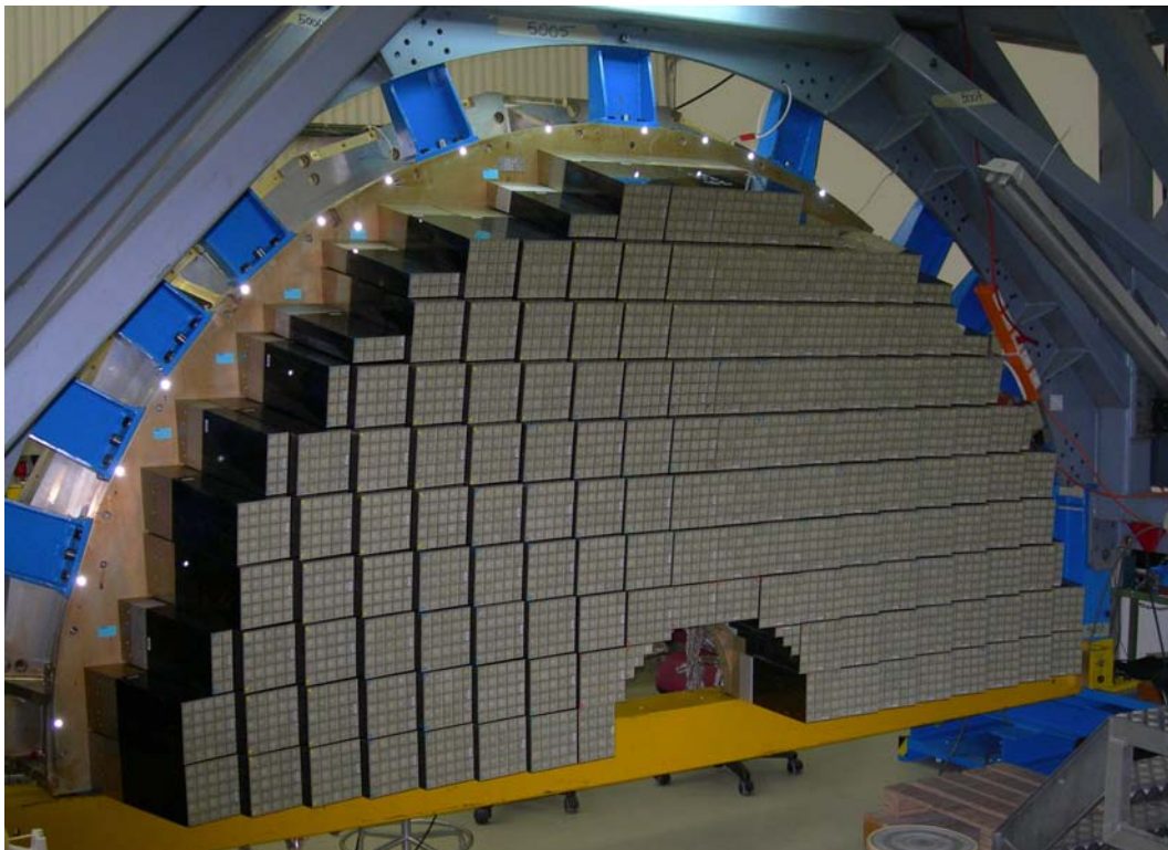
Figure 4.7: An endcap Dee, fully equipped with supercrystals.
