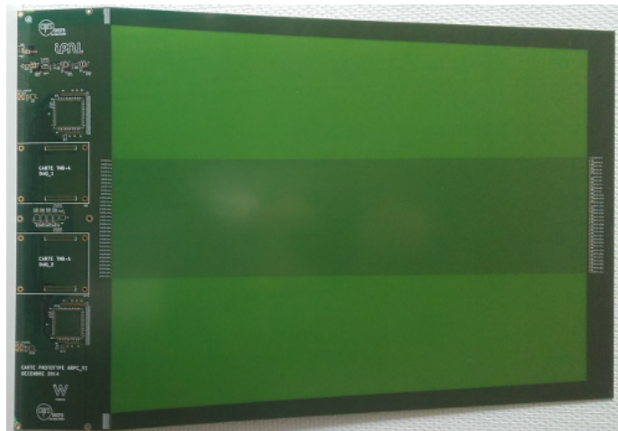
Figure 7. Picture of a strip board designed for a RE1/1 station using 16-channel PETIROC ASICs and 25 ns TDC.
